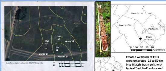
Location of Cedar Run 3 site (right), 3 monitoring sites above and map of preexisting soils (above). Created wetlands at CR 3 were excavated 25 to 50 cm into Triassic Basin soils with typical "red bed" colors and strong subsoil shrink-swell potential. One profile shown above center.
