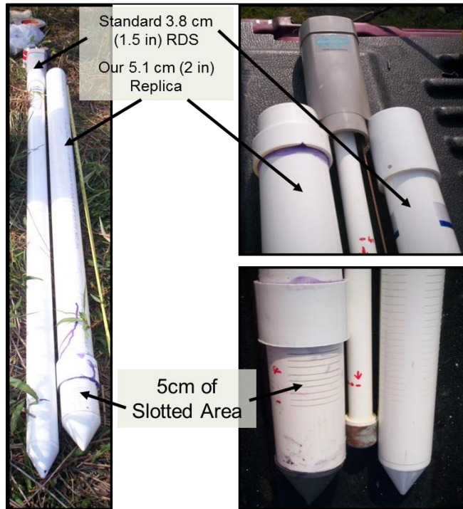
Figure 10. Middle-depth piezometer and standard well with the RDS sensor at the Cedar Run Site.
