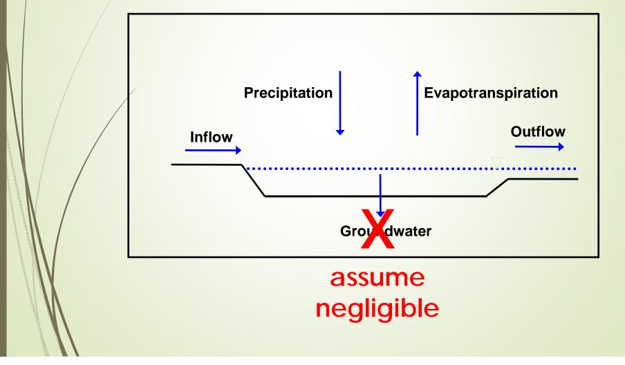
A "simple" way to create a mitigation wetland is to create a perched system Can work on hilltops with low permeability compacted subsoils
