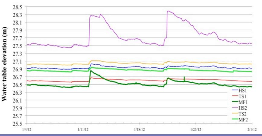
Bold green lines represent wells screened in fine-grained sediment. Their synchronicity with other wells suggests macropores in these sediments enhance vertical connectivity between coarse and fine units.
