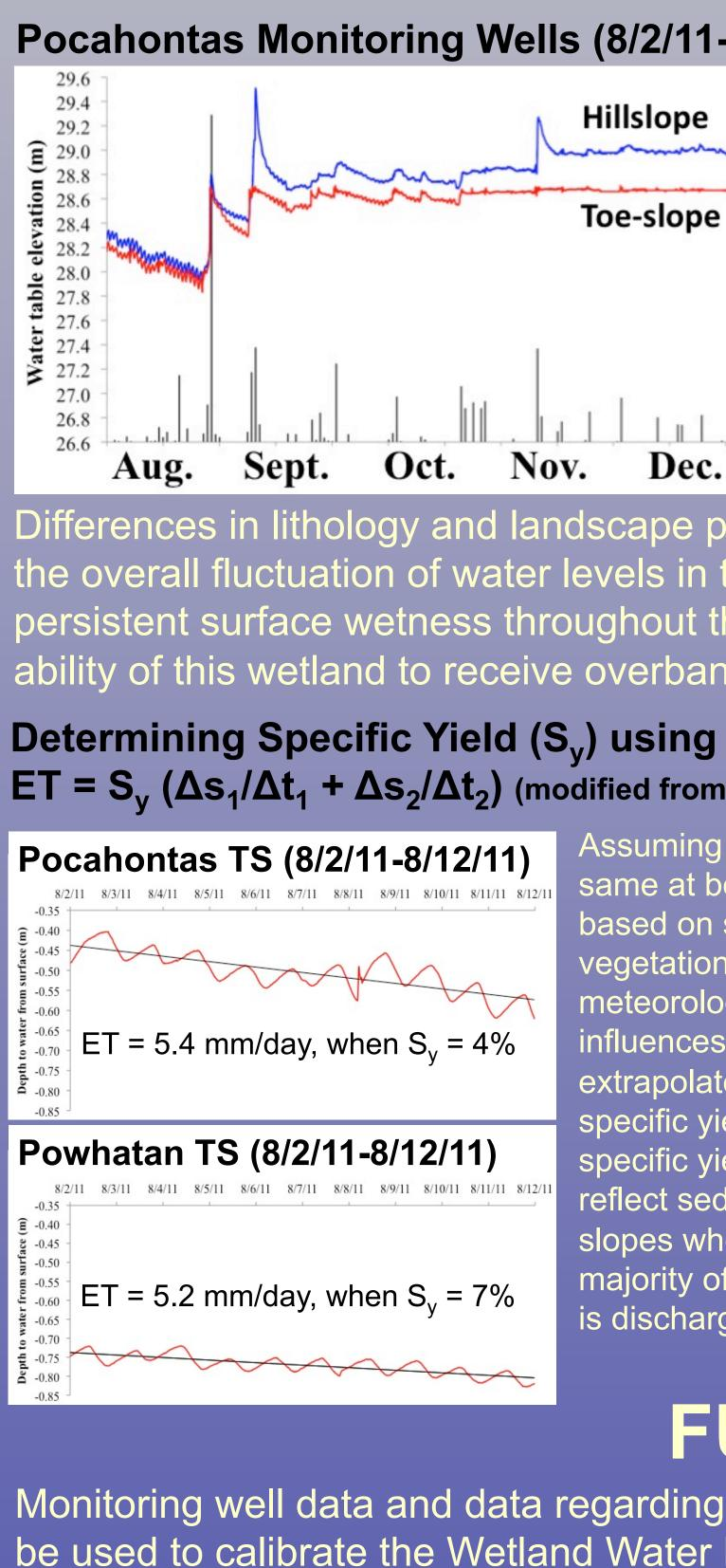
Monitoring well data and data regarding the hydrologic properties of surface materials in these settings will be used to calibrate the Wetland Water Budget model, which will calculate water budgets for a planned wetland site on Piedmont floodplains or terraces using many possible water sources. Historical maps and land-use records will be obtained to constrain the time frame and depositional environment for each site.
