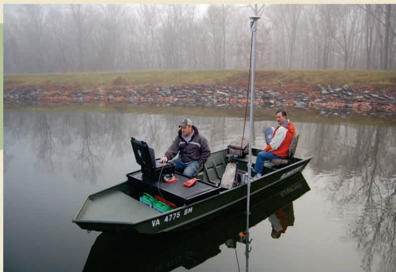
Bathymetric Survey using the Echotrac System
