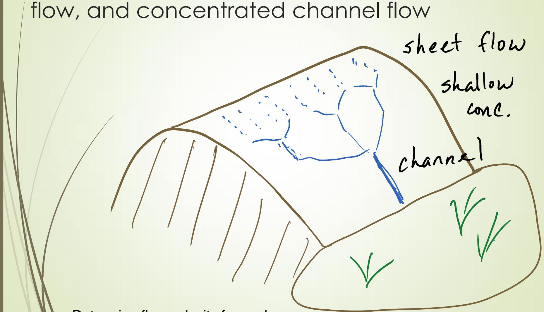
Determine flow velocity for each type of flow and divide flow distance by flow velocity to get travel time.
