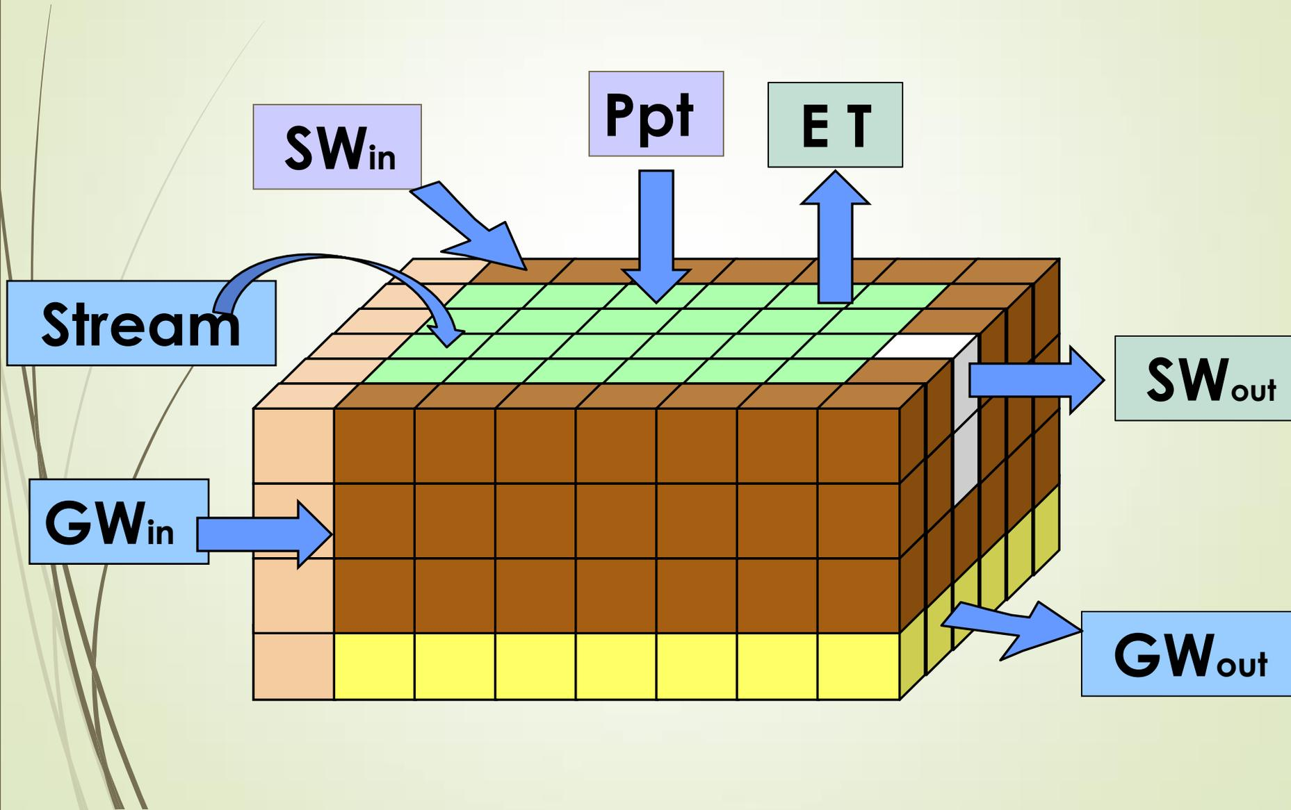
The Advanced model determines daily flow rates between cells/boxes using Darcy's law and then determines volume of water in the cell for that day
