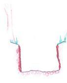
**POOR:** This channel is similarly incised as the 'Severe' Channel Condition with <u>vertical and/or lateral instability</u>, channel invert is below the average rooting depth within the banks and the majority of both banks are vertical or undercut.
