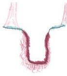
**SEVERE:** This channel is deeply incised with <u>vertical and/or lateral instability</u> and will likely continue to widen or incise. The channel invert is below the average rooting depth within the banks and the majority of both banks are vertical or undercut.
