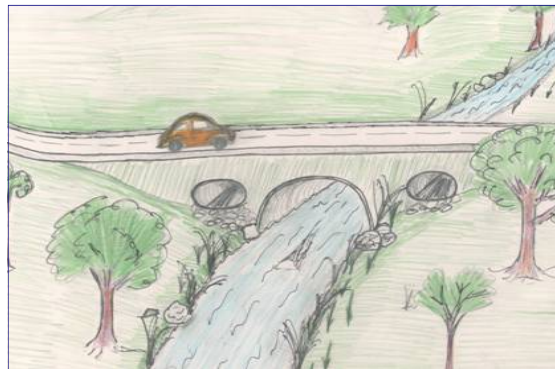
NEGLIGIBLE - Con/Span or Bottomless culvert with flanking culverts for floodplain conveyance. Only temporary impacts to Waters of the U.S. during construction.
