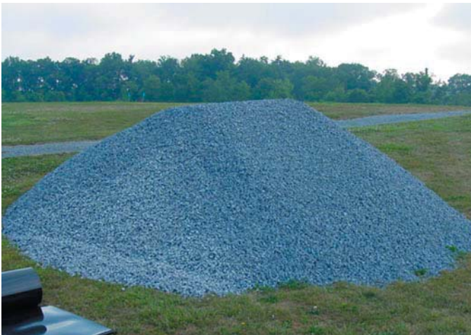
Fig. 1.9 Gravel used under traditional porous asphalt system.
