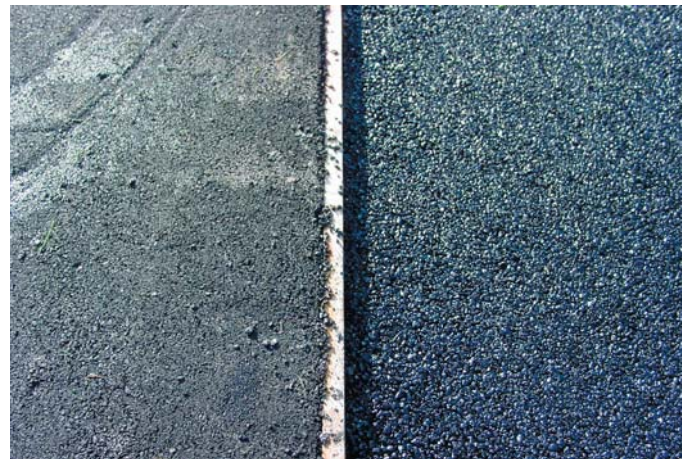
Fig. 1.7 A comparison of traditional asphalt (left) and porous asphalt (right) when dry. The gaps in the porous asphalt make it appear more coarse and unfinished.
