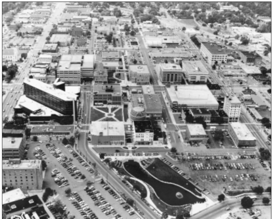
The daylighted section of Arcadia Creek, beginning near the top center of this photograph, runs through three full city blocks in downtown Kalamazoo, Michigan, then opens into a stormwater pond. Courtesy of STS Consultants, Ltd.
