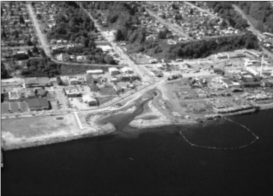
The newly recreated estuary of Valley Creek in Port Angeles, Washington. The project used excavation spoils from the estuary to fill the K-Ply mill's log pond, once located where the log piles lie between the estuary and the mill. Courtesy of Port of Port Angeles.
