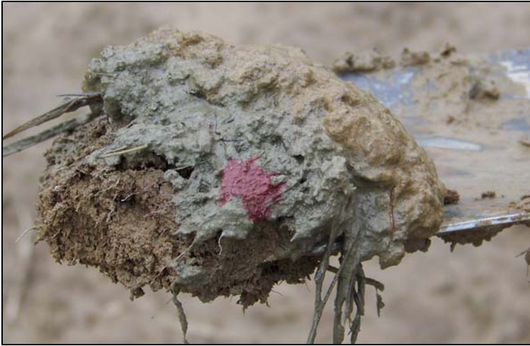
Figure 57. When alpha, alpha-dipyridyl dye is applied to a soil containing reduced iron, a positive reaction is indicated by a pink or red coloration to the treated area.
