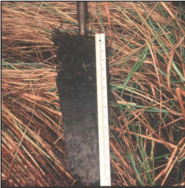
Figure 15. The mucky modified sandy layer is approximately 3 in. (7.5 cm) thick. Scale in inches on the right side of ruler.
