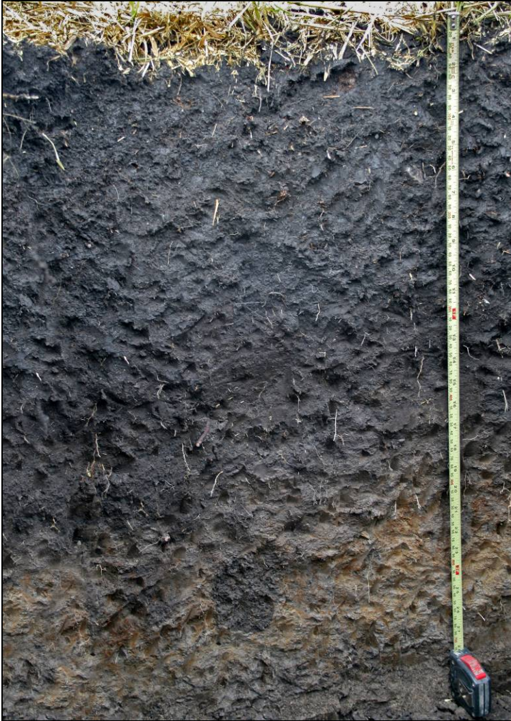
Figure 14. Deep observations may be necessary to identify the depleted or gleyed matrix below a thick, dark surface layer. In this example, the depleted matrix starts at 20 in. (50 cm).
