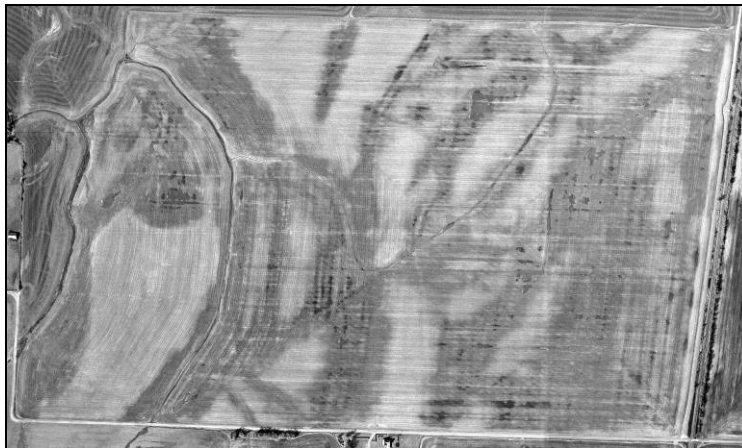
Figure 61. Aerial photograph of an agricultural field with saturated soils indicated by darker colors.
