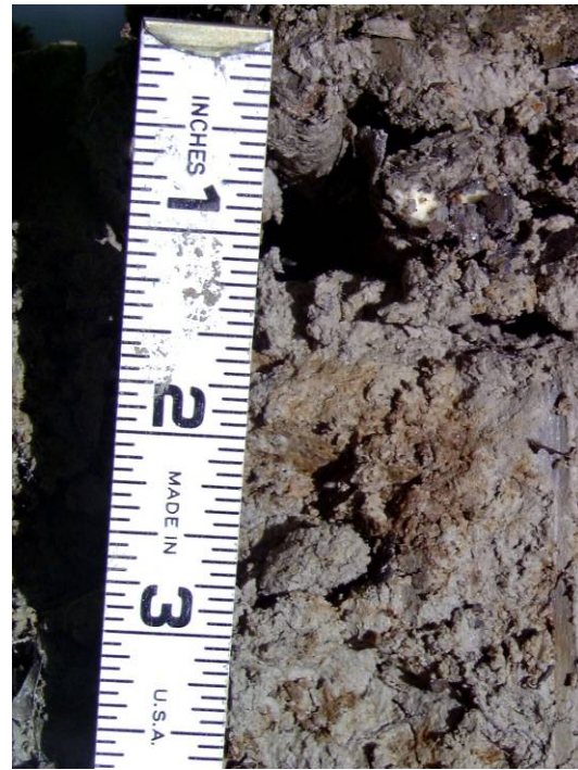
Figure 25. Redox concentrations at 2 in. (5 cm)
