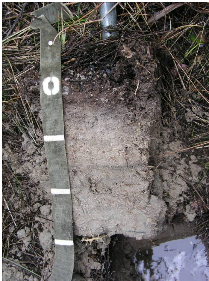
Figure 68. Soil with a mucky-peat surface over sand. Increments on tape are 4 in. (10 cm).
