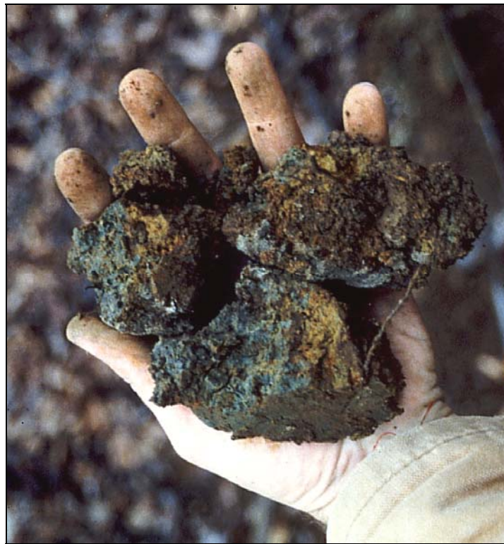
Figure 66. Non-hydric soils that are high in glauconite can have colors similar to hydric soils. In hydric soils, glauconite can mask redoximorphic features.
