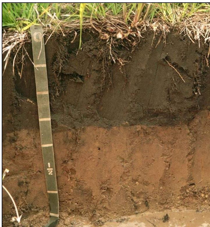
Figure 69. An anomalous bright sandy soil. This example has a relatively thick surface layer. Scale in 4-in. (10-cm) increments.
