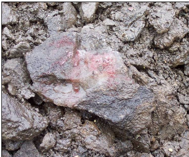
Figure 58. When alpha, alpha-dipyridyl dye is applied to a soil containing reduced iron, a positive reaction is indicated by a pink or red coloration to the treated area.
